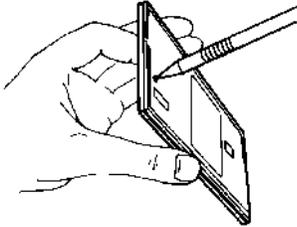
1) With a pencil or straightened paper clip and the calculator ON, push the "ALL RESET" button on the left side of the back of the calculator. (There may be a white label covering the "ALL RESET" button. If so, gently lift up the lower left corner of the label to reveal the "ALL RESET" button.) You should see 4 stars in the display (2 on the left, 2 on the right).
