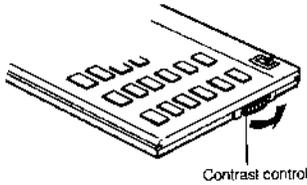
The calculator is equipped with a control to adjust the contrast of the LCD (liquid crystal display). As the batteries age, the contrast will need to be adjusted from time to time. Adjust the display contrast with the knob on the right-hand end of the computer (under the On/Off switch). While looking at the display from a position about 70 degrees above the keyboard, first increase the contrast until black squares are clearly visible behind the
