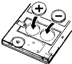
4) Slide the silver-colored battery compartment cover upward to open the compartment; remove the cover. The batteries are now disconnected; remove and discard them.
